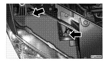
3. Rotate bulb and connector ¼ turn and pull outward from assembly.
